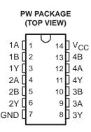
The SN74LV86A is a quadruple 2-input exclusive-OR gate designed for 2-V to 5.5-V V<sub>CC</sub> operation.
