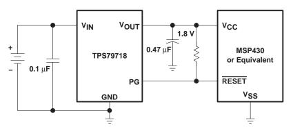
Figure 15. MSP430 Microcontroller Powered by the TPS79718 Regulator
