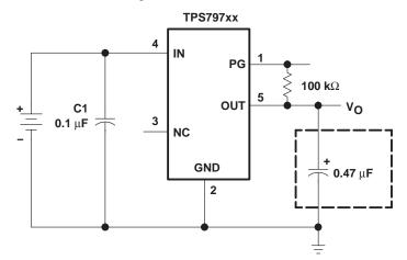
Figure 14. Typical Application Circuit
