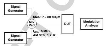
Figure 17. 1% Cross Modulation Distortion Measurement Circuit
