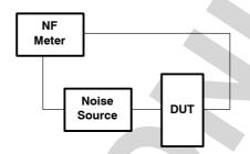
Figure 16. Noise Figure Measurement Circuit
