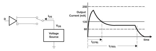
Figure 8. Driver Short-Circuit Test Circuit and Waveforms (Short Circuit applied at Time t = 0)
