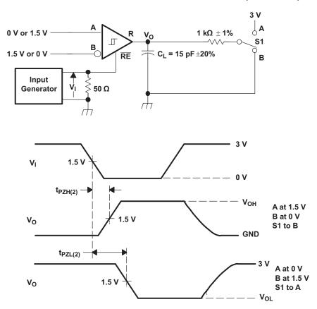
Figure 12. Receiver Enable Time From Standby (Driver Disabled)
