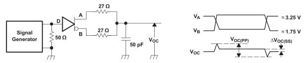
Figure 5. Driver V<sub>OC</sub> Test Circuit and Waveforms
