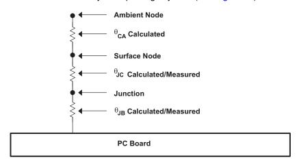
Figure 21. Thermal Resistance
