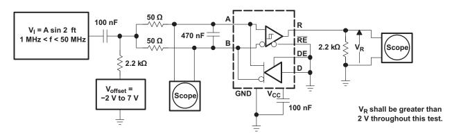
Figure 11. Receiver Common-Mode Rejection Test Circuit
