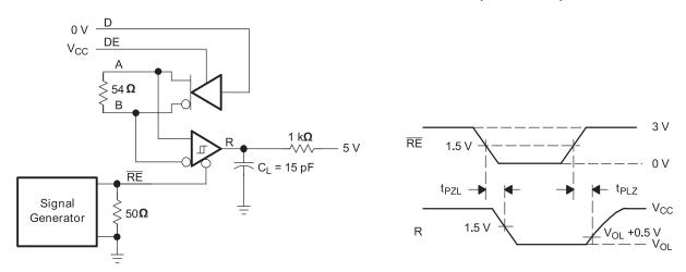
Figure 14. Receiver Enable Test Circuit and Waveforms, Data Output Low (Driver Active)
