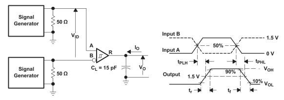
Figure 10. Receiver Switching Test Circuit and Waveforms
