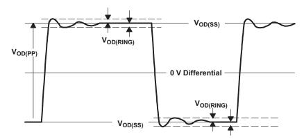
(1)  $V_{OD(RING)}$  is measured at four points on the output waveform, corresponding to overshoot and undershoot from the  $V_{OD(H)}$  and  $V_{OD(L)}$  steady state values.
