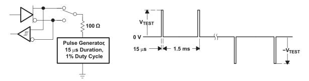
Figure 15. Test Circuit and Waveforms, Transient Overvoltage Test
