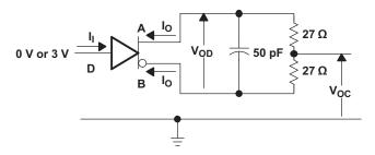
Figure 1. Driver Test Circuit, V<sub>OD</sub> and V<sub>OC</sub> Without Common-Mode Loading
