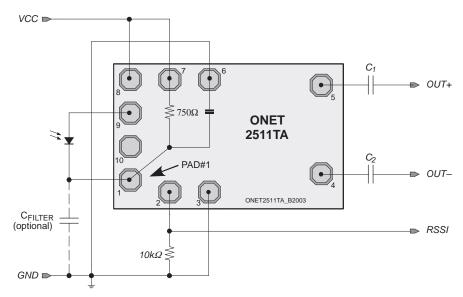
Figure 3. Basic Application Circuit
