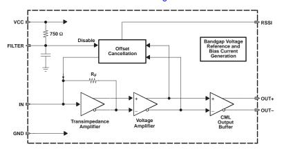
Figure 1. Simplified Block Diagram of the ONET2511TA
