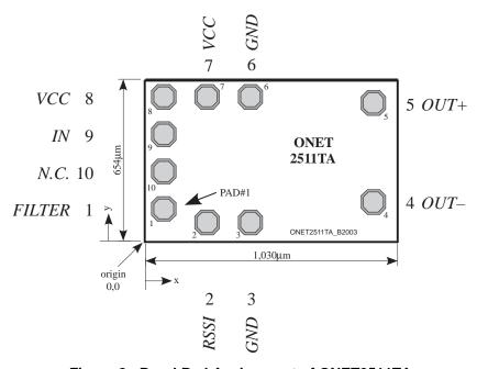
Figure 2. Bond Pad Assignment of ONET2511TA
