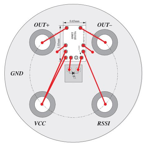
Figure 6. TO46 Layout Example Using the ONET2511TA
