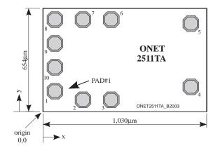
Figure 4. Chip Dimensions and Pad Locations
