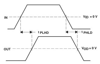
Figure 6. Propagation Delay Input to Output
