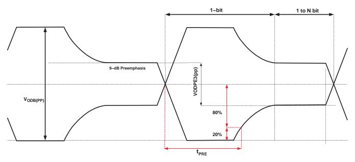
Figure 4. t<sub>(PRE)</sub> Preemphasis Duration Measurement
