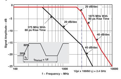
Figure 17. Approximate Frequency Spectrum of the Transmit Output Signal With 80 ps Rise Time
