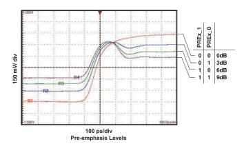
NOTE: 51 Inch (128.54 cm) Input Trace, dR = 4.25 Gbps; 2<sup>7-1</sup> PRBS **Figure 9. Data Input and Output Pattern**
