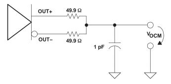
Figure 2. Common-Mode Output Voltage Test Circuit
