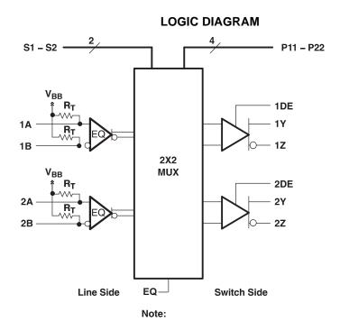
V<sub>BB</sub>: Receiver input internal biasing voltage (allows ac coupling)
