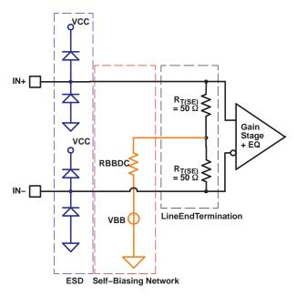
Figure 1. Equivalent Input Circuit Design
