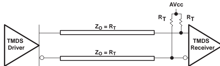
Figure 3. Typical Termination for TMDS Output Driver
