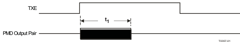
Figure 9-17. 10Mb/s Jabber Timing
