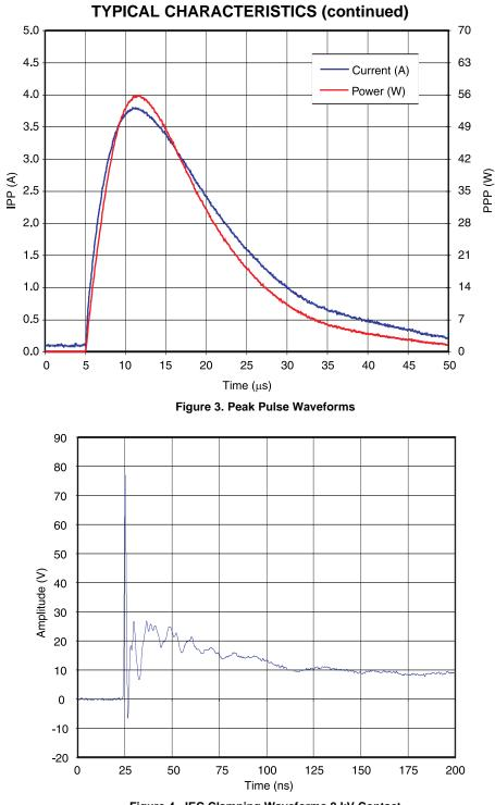
Figure 4. IEC Clamping Waveforms 8 kV Contact
