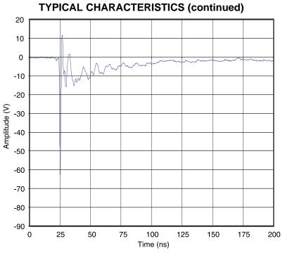
Figure 5. IEC Clamping Waveforms -8 kV Contact
