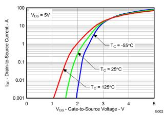
Figure 3. Transfer Characteristics
