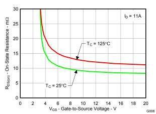
Figure 7. On-State Resistance vs. Gate-to-Source Voltage
