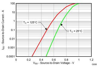
Figure 9. Typical Diode Forward Voltage
