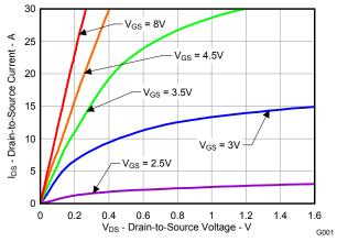
Figure 2. Saturation Characteristics
