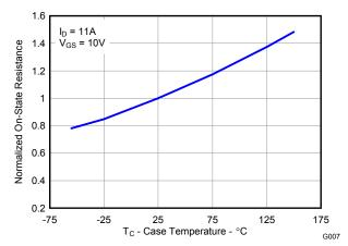
Figure 8. Normalized On-State Resistance vs. Temperature
