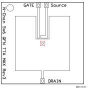
Max  $R_{\theta JA} = 51^{\circ} C/W$  when mounted on 1 inch² (6.45 cm²) of 2-oz. (0.071-mm thick) Cu.
