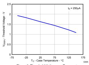
Figure 6. Threshold Voltage vs. Temperature
