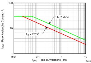
Figure 11. Single Pulse Unclamped Inductive Switching
