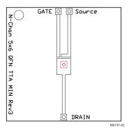
Max  $R_{\theta JA} = 131^{\circ} C/W$  when mounted on a minimum pad area of 2-oz. (0.071-mm thick) Cu.
