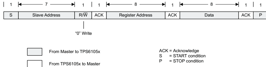
Figure 46. Write Data Transfer Format in F/S-Mode
