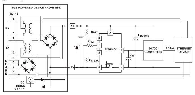
Figure 1. For Applications 40 V < V<sub>IN</sub> < 57 V.
