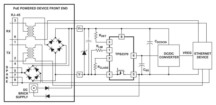
Figure 2. For Applications  $V_{IN}$  < 40 V.
