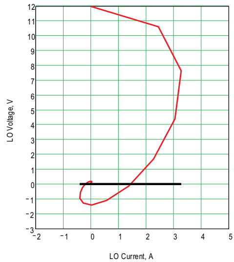
Figure 25. Turn-Off Voltage and Current Switching Diagram
