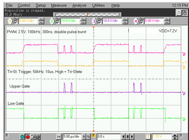
Figure 21. 2.5-V Amplitude PWM Pulse
