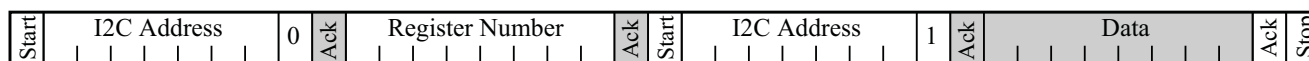
Figure 31. Format of a Register Read. Shaded Regions Denote Bus Control by TPS2358/9
