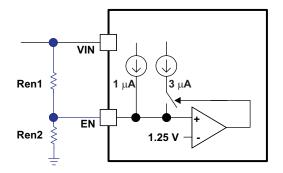
Figure 11. Adjustable Input Undervoltage Lockout
