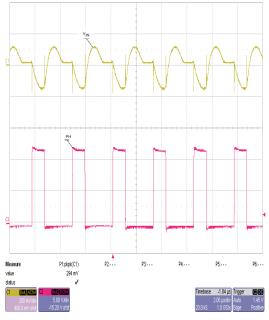
Figure 20. TPS54233 Input Ripple
