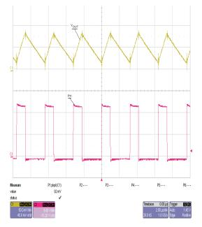
Figure 21. TPS54233 Output Ripple
