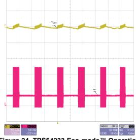
Figure 24. TPS54233 Eco-mode<sup>™</sup> Operation
