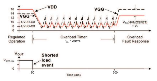
Figure 32. Overload Behavior with a Shorted Output
