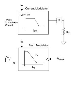
Figure 25. Modulation Control Blocks
