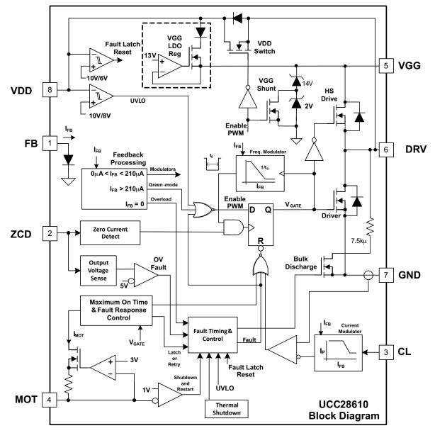
Figure 19. Symplified Block Diagram
