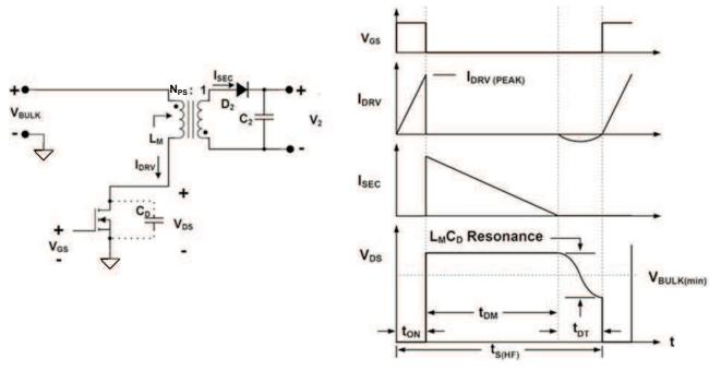
Figure 20. Basic Flyback Converter and Waveforms at Peak Load and Minimum V<sub>BULK</sub> Voltage
