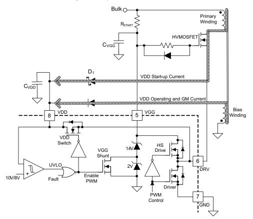
Figure 22. Start-Up Currents for the Cascode Architecture
