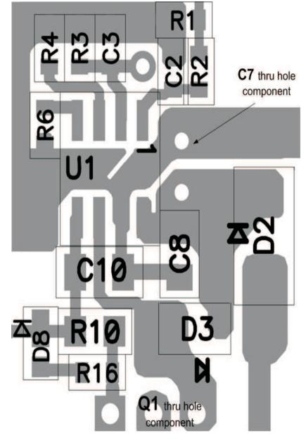
Figure 36. Typical Layout of the Device on a Single Layer PCB
