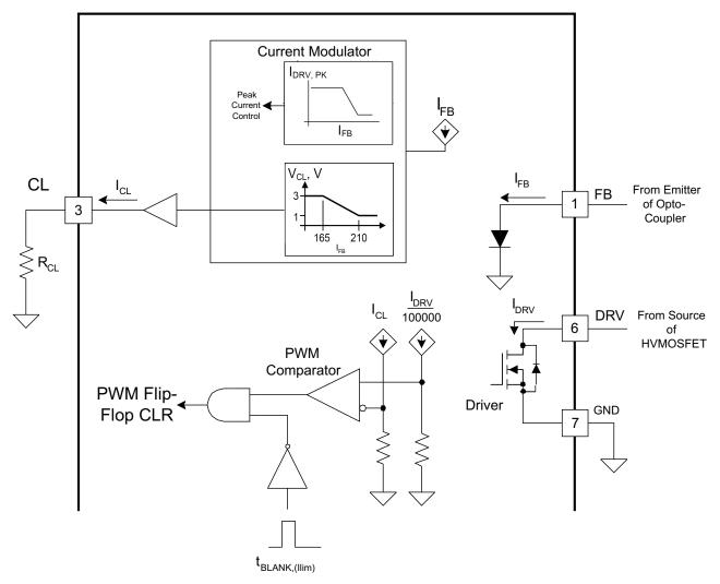
Figure 27. CL pin and DRV Current Sense
