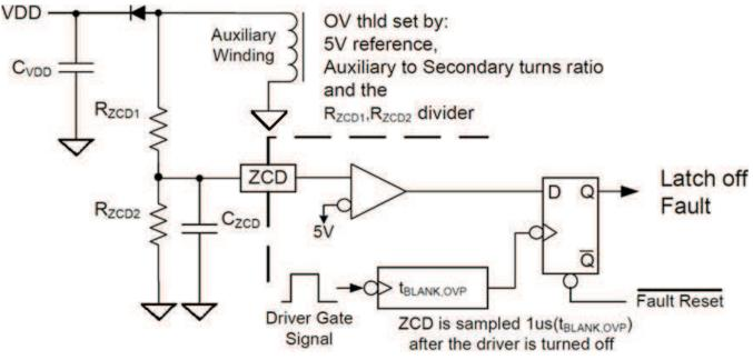
Figure 34. Output Over-Voltage Protection with ZCD Pin
