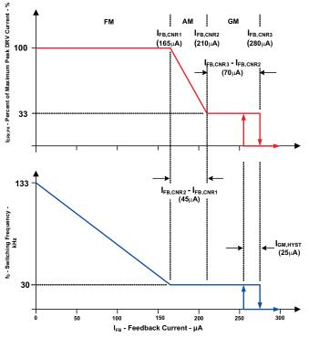
Figure 26. Control Diagram with Operating Modes
