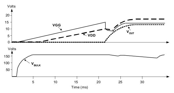
Figure 23. Typical Start-Up Waveforms for a 17-V Bias Winding Voltage
