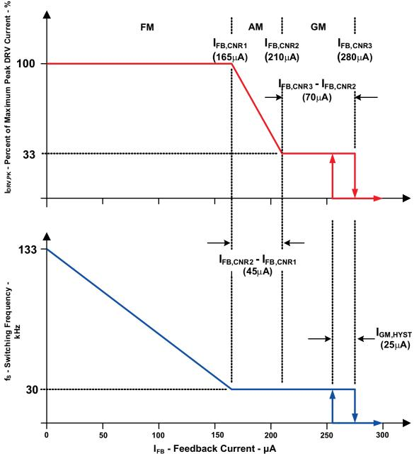
Figure 2. FB Electrical Condition Detail
