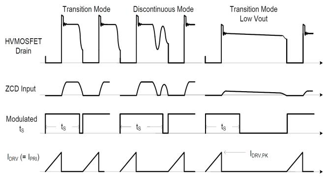
Figure 28. Switching Cycle Waveforms
