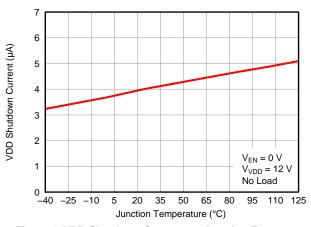
Figure 4. VDD Shutdown Current vs. Junction Temperature
