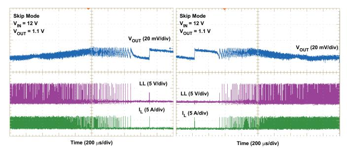
Figure 27. CCM to DCM Transition Waveforms
