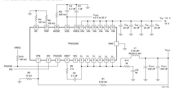
Figure 1. Typical Application Circuit Diagram
