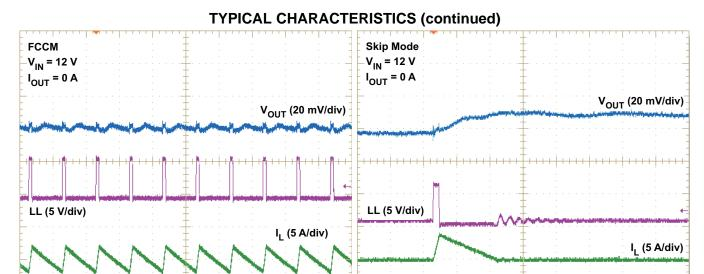
Figure 25. 1.1-V Output FCCM Mode Steady-State Operation
