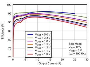
Figure 16. Efficiency vs Output Current
