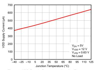
Figure 3. VDD Supply Current vs. Junction Temperature
