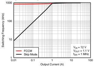
Figure 9. Switching Frequency vs. Output Current
