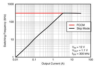
Figure 7. Switching Frequency vs. Output Current
