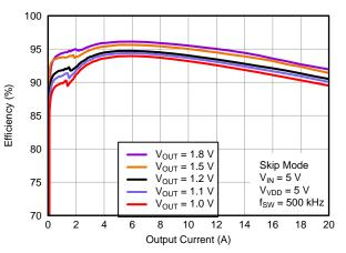
Figure 20. Efficiency vs Output Current
