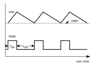
Figure 36. On-Time Control Without Ramp Compensation
