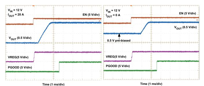
Figure 21. Start-Up Waveforms
