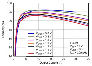
Figure 15. Efficiency vs Output Current
