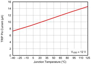
Figure 5. TRIP Pin Current vs. Junction Temperature
