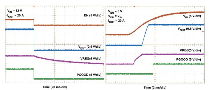
Figure 23. Shutdown Waveforms
