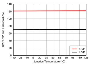
Figure 6. OVP/UVP Trip Threshold vs. Junction Temperature
