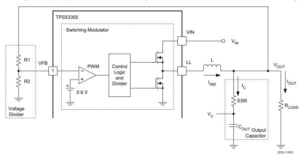
Figure 38. Simplified Modulator Model
