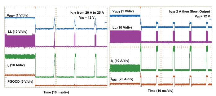
Figure 31. Overcurrent Protection Waveforms
