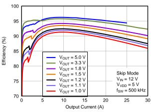
Figure 18. Efficiency vs Output Current
