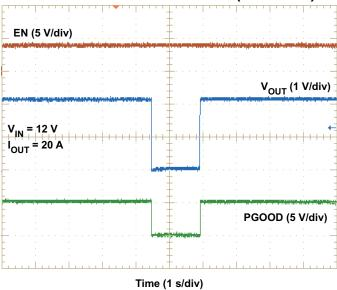
Figure 33. Over-temperature Protection Waveforms
