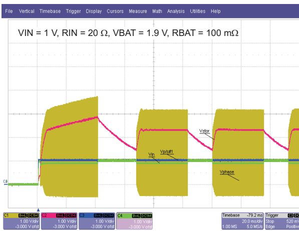
Figure 20. Example of Startup When VBAT is Held Below UV Setting
