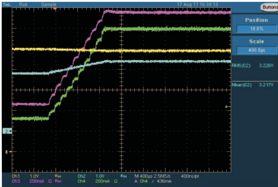
Figure 11. Charge Current Response – 550mA to 1.55A CH1: VIN, CH2: VBAT, CH3: IBAT, CH4: IVIN
