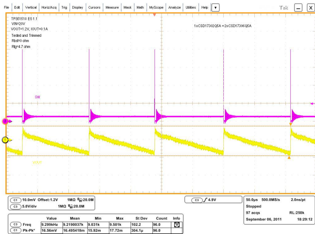
Figure 15. Steady-State Ripple, I LOAD = 0.1 A
