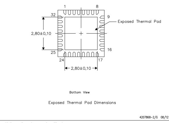
NOTE: All linear dimensions are in millimeters
