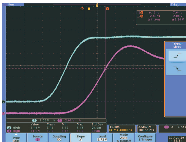
Figure 26. Typical Turnoff Waveform (VDD = 10 V, C L = 1 nF)
