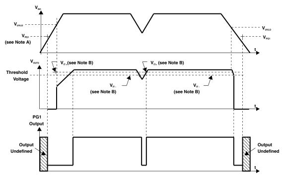
NOTES: A.  $V_{PG}$  is the minimum input voltage for a valid PG. The symbol  $V_{PG}$  is not currently listed within EIA or JEDEC standards for semiconductor symbology.
