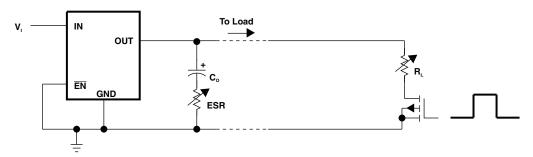
Figure 30. Test Circuit for Typical Regions of Stability
