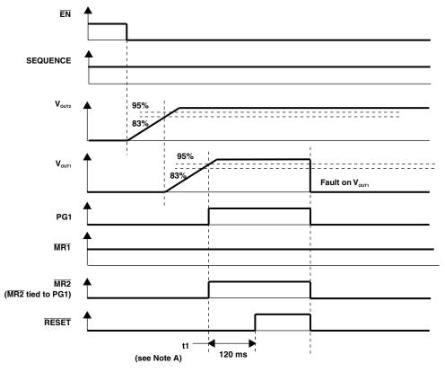
NOTE A: t1 - Time at which both  $V_{\text{out1}}$  and  $V_{\text{out2}}$  are greater than the PG thresholds and  $\overline{\text{MR1}}$  is logic high.
