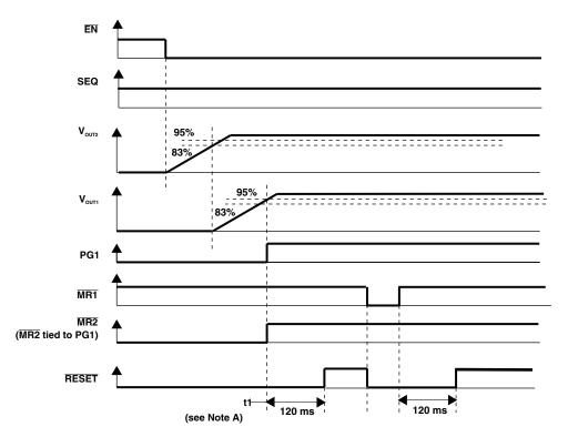
NOTE A: t1 - Time at which both  $V_{\text{OUT}1}$  and  $V_{\text{OUT}2}$  are greater than the PG thresholds and  $\overline{\text{MR1}}$  is logic high.
