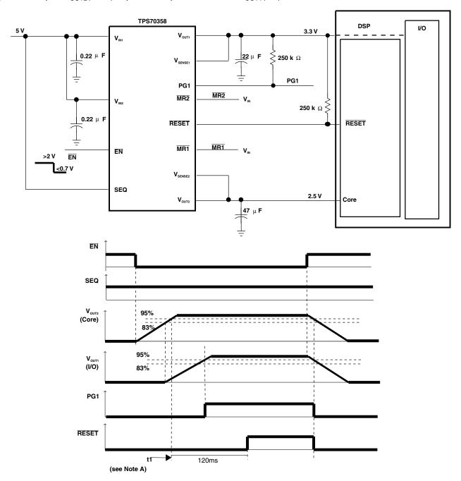
NOTE A: t1 - Time at which both  $V_{\text{OUT1}}$  and  $V_{\text{OUT2}}$  are greater than the PG1 thresholds and  $\overline{\text{MR1}}$  is logic high.
