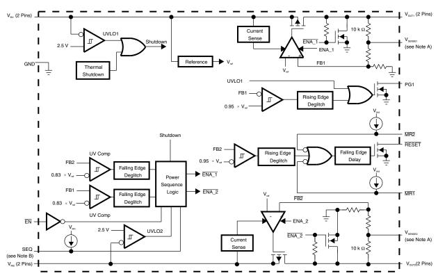
NOTES: A. For most applications, V<sub>SENSE1</sub> and V<sub>SENSE2</sub> should be externally connected to V<sub>OUT</sub> as close as possible to the device. For other implementations, refer to SENSE terminal connection discussion in the Application Information section. B. If the SEQ terminal is floating at the input, V<sub>OUT2</sub> powers up first.
