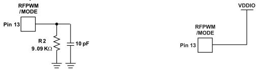
Figure 16. Programmable Dimming Mode Selection Figure 17. Direct PWM Dimming Mode Selection
