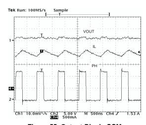
Figure 55. Output Ripple CCM
