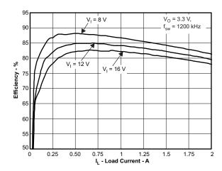
Figure 61. Efficiency vs Load Current
