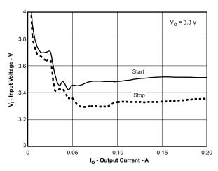
Figure 26. 3.3-V Start/Stop Voltage
