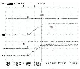
Figure 53. Startup With EN
