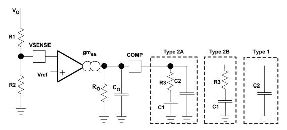
Figure 49. Types of Frequency Compensation
