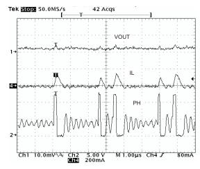
Figure 57. Output Ripple, PSM
