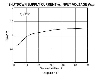
VIN SUPPLY CURRENT vs INPUT VOLTAGE
