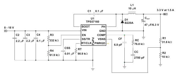
Figure 51. High Frequency, 3.3-V Output Power Supply Design with Adjusted UVLO
