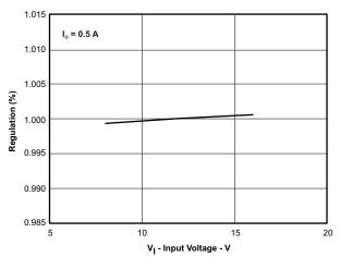
Figure 64. Regulation vs Input Voltage
