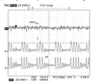
Figure 25. Pulse Skip Mode Operation
