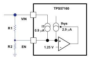
Figure 28. Adjustable Undervoltage Lockout (UVLO)
