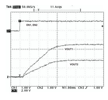
Figure 35. Ratiometric Startup Using Coupled SS/TR Pins
