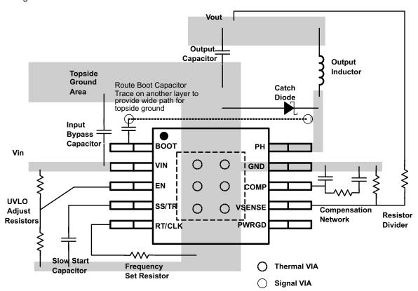
Figure 65. PCB Layout Example
