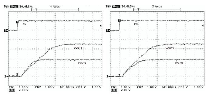
Figure 37. Ratiometric Startup With  $V_{OUT2}$  Leading  $V_{OUT1}$
