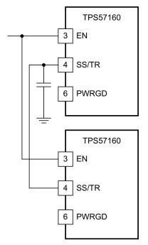
Figure 34. Schematic for Ratiometric Start-Up Using Coupled SS/TR Pins
