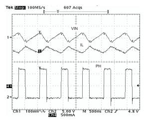
Figure 58. Input Ripple CCM
