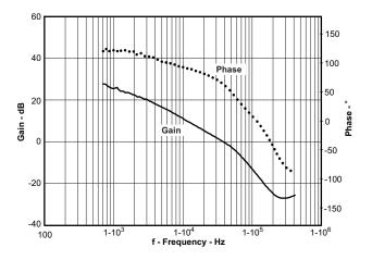
Figure 62. Overall Loop Frequency Response
