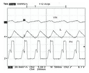
Figure 59. Input Ripple DCM
