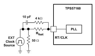
Figure 43. Synchronizing to a System Clock
