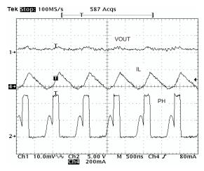
Figure 56. Output Ripple, DCM
