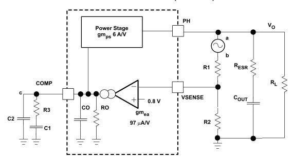
Figure 47. Small Signal Model for Loop Response
