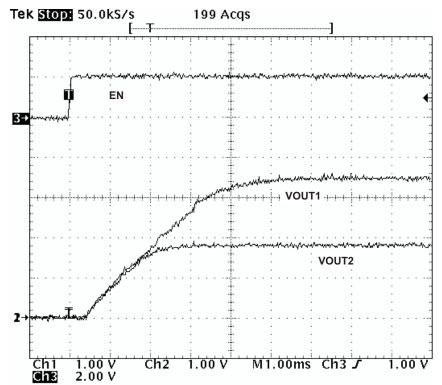
Figure 39. Simultaneous Startup With Tracking Resistor
