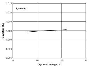
Figure 64. Regulation versus Input Voltage
