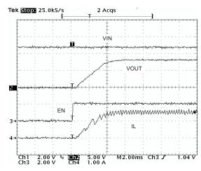
Figure 53. Startup With EN
