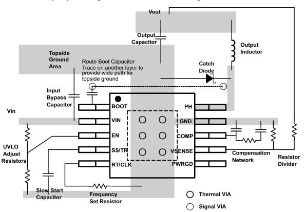
Figure 65. PCB Layout Example
