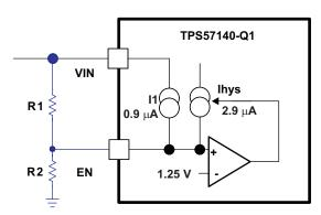
Figure 28. Adjustable Undervoltage Lockout (UVLO)
