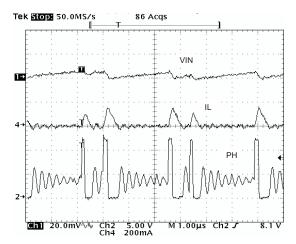
Figure 60. Input Ripple, PSM
