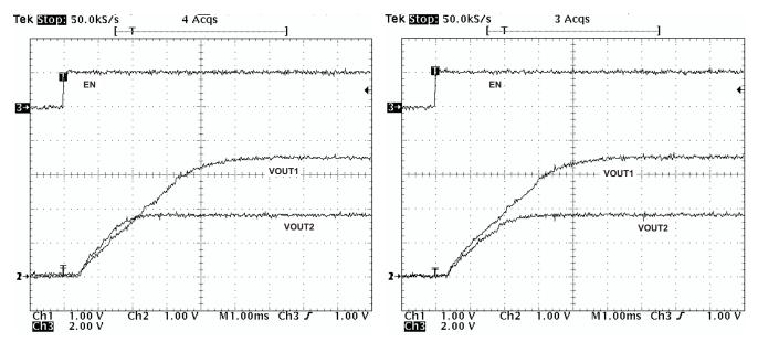
Figure 37. Ratiometric Start-Up With  $V_{\text{OUT2}}$  Leading Figure 38. Ratiometric Start-Up With  $V_{\text{OUT1}}$  Leading  $V_{\text{OUT2}}$
