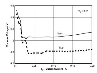
Figure 27. 5-V Start and Stop Voltage
