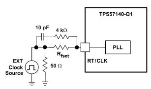
Figure 43. Synchronizing to a System Clock
