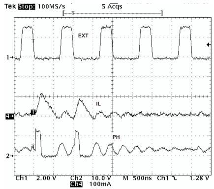
Figure 46. Plot of Synchronizing in PSM
