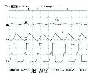
Figure 59. Input Ripple, DCM
