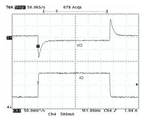
Figure 52. Load Transmit
