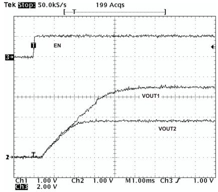
Figure 39. Simultaneous Start-Up With Tracking Resistor
