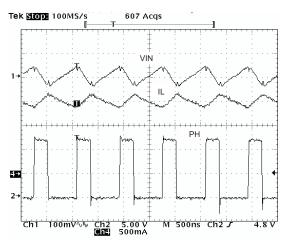
Figure 58. Input Ripple, CCM
