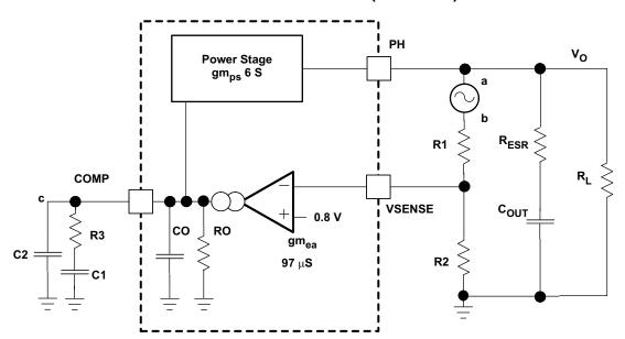
Figure 47. Small-Signal Model for Loop Response
