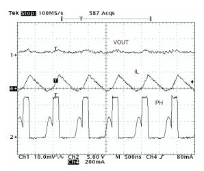
Figure 56. Output Ripple, DCM
