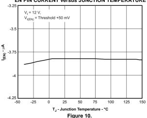
**EN PIN CURRENT versus JUNCTION TEMPERATURE**
