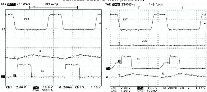
Figure 44. Plot of Synchronizing in CCM
