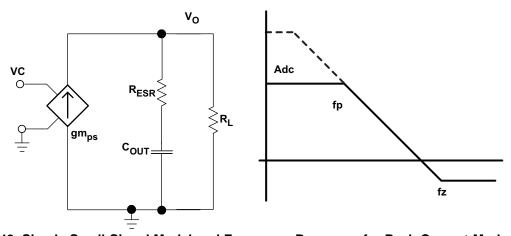
Figure 48. Simple Small-Signal Model and Frequency Response for Peak-Current-Mode Control
