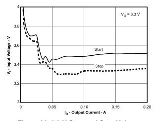
Figure 26. 3.3-V Start and Stop Voltage
