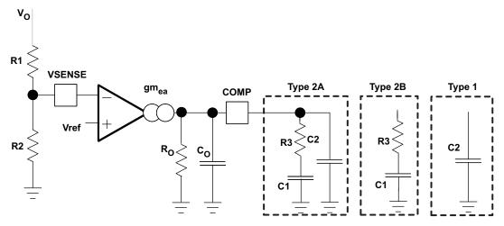
Figure 49. Types of Frequency Compensation
