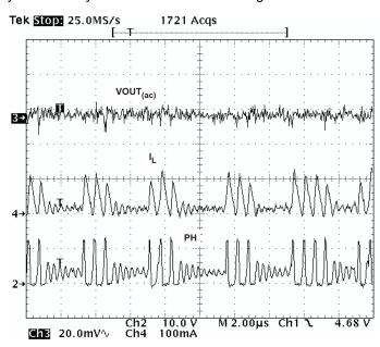
Figure 25. Operation in Pulse-Skip Mode
