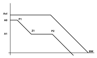
Figure 50. Frequency Response of the Type 2A and Type 2B Frequency Compensation
