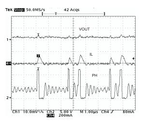
Figure 57. Output Ripple, PSM
