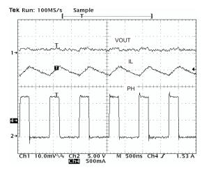
Figure 55. Output Ripple, CCM
