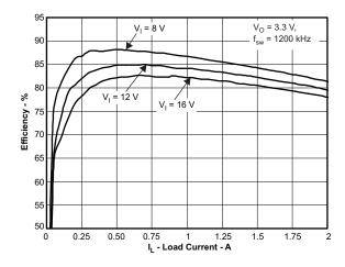
Figure 61. Efficiency versus Load Current
