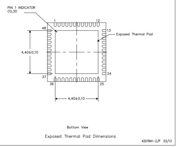
NOTE: All linear dimensions are in millimeters
