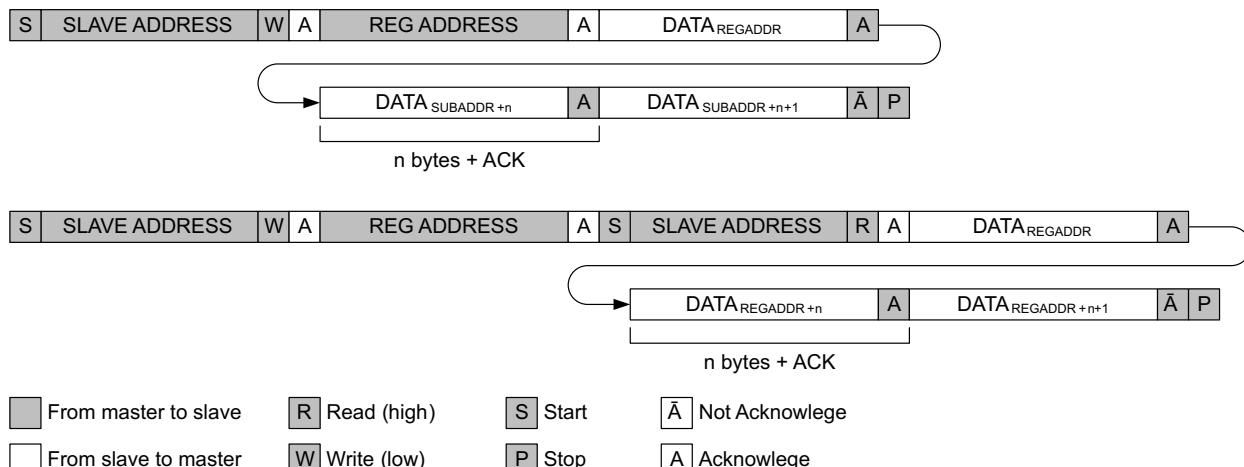
Figure 20. I<sup>2</sup>C Data Protocol. TOP: Master writes data to slave. BOTTOM: Master reads data from slave.
