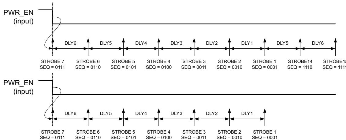
**Figure 3. Power-Down Sequence Follows Reverse Power-Up Sequence. TOP: Power-down sequence from ON state to OFF state (all rails are turned OFF). BOTTOM: Power-down sequence from ON state to SLEEP state. STROBE14 and 15 are omitted to allow LDO1/2 to remain ON.**
