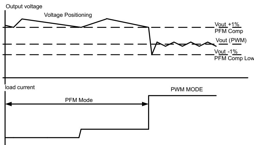
**Figure 15. Dynamic Voltage Positioning in Power Save Mode**
