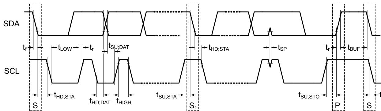
Figure 22. I<sup>2</sup>C Data Transmission Timing
