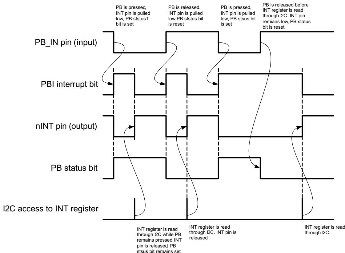
**Figure 5. Timing Diagram of the Push-Button Monitor Circuit**
