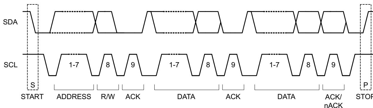
Figure 21. I<sup>2</sup>C Start/Stop/Acknowledge Protocol
