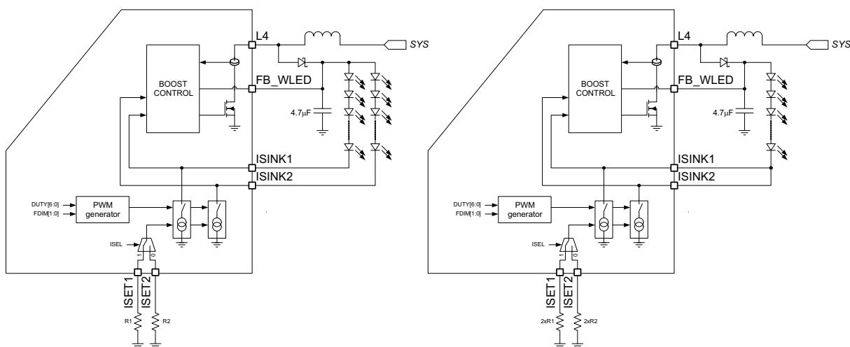
**Figure 17. Block Diagram of WLED Driver. LEFT: Dual string operation. RIGHT: Single string operation (same LED current as dual string). Note that for single string operation both ISINK pins are shorted together and RSET values are doubled.**
