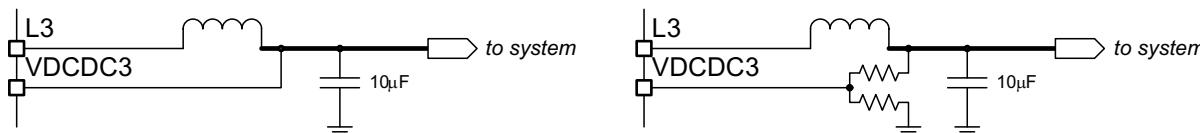
**Figure 14. DCDC1, 2, and 3 Offer Two Methods to Adjust the Output Voltage. Example for DCDC3. LEFT: fixed voltage options programmable through I<sup>2</sup>C (XADJ3 = 0, default). RIGHT: Voltage is set by external feedback resistor network (XADJ3 = 1).**
