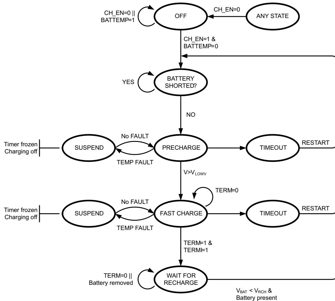
Figure 11. State Diagram of Battery Charger
