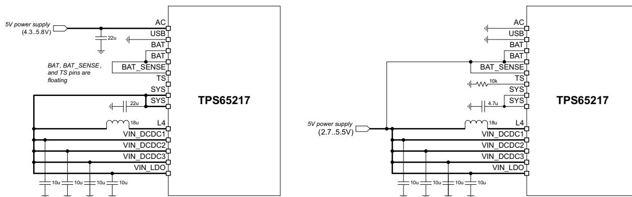
**Figure 18. Left: Power-connection for battery-less/5-V only operation. The SYS node and DCDC converters are protected against input over-voltage up to 20 V. Right: Power-connection for 5-V only operation. The DCDC converters are not protected against input over-voltage, but power-efficiency is higher because the internal power-path switches are bypassed.**
