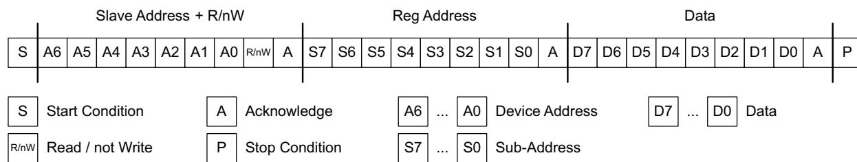
**Figure 19. Sub-Address in I<sup>2</sup>C Transmission**
