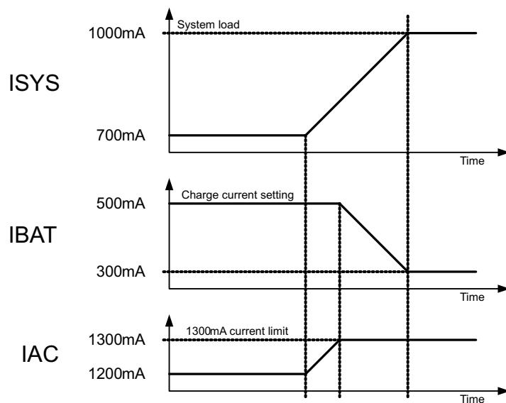
**Figure 9. Power Path Management.** In this example the AC input current limit is set to 1300 mA, battery charge current is 500 mA and system load is 700 mA. As the system load increases to 1000 mA battery charging current is reduced to 300 mA to maintain AC input current of 1300 mA.
