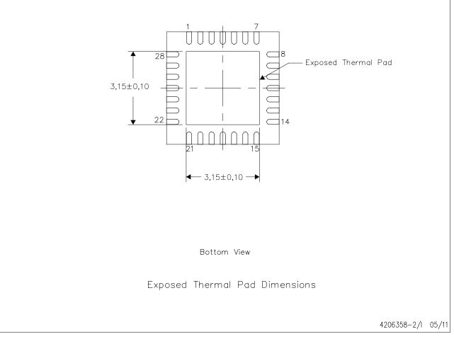
NOTE: All linear dimensions are in millimeters
