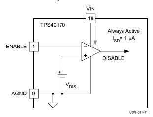
Figure 17. TPS40170 ENABLE Functional Block
