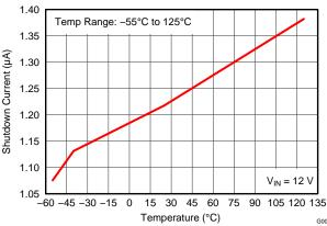
Figure 6. Shutdown Current vs Junction Temperature
