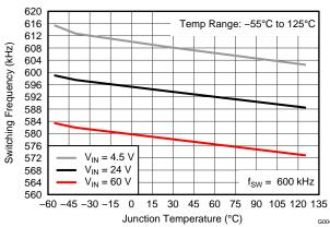
Figure 5. Switching Frequency vs Junction Temperature ( $f_{\rm SW} = 600~{\rm kHz}$ )
