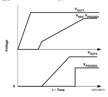
Figure 32. Sequential Start-Up Schematic
