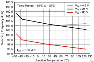
Figure 3. Switching Frequency vs Junction Temperature (f<sub>SW</sub> = 100 kHz)
