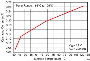
Figure 7. Operating Current vs Junction Temperature
