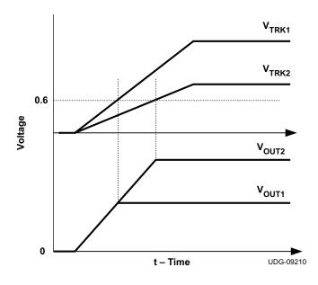
Figure 29. Simultaneous Voltage-Tracking Waveform
