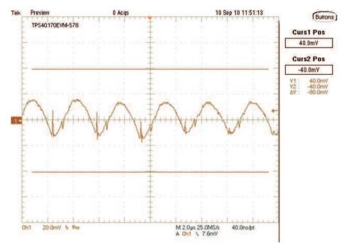
Figure 38. Output Ripple Waveform
