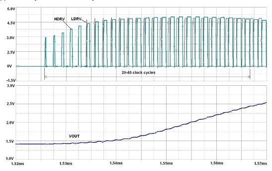
Figure 34. Start-Up Switching Waveform During Pre-Biased Condition
