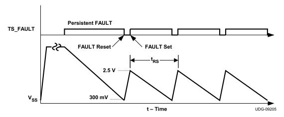
Figure 24. Overtemperature Fault Restart Timing
