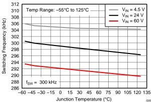
Figure 4. Switching Frequency vs Junction Temperature (f<sub>SW</sub> = 300 kHz)
