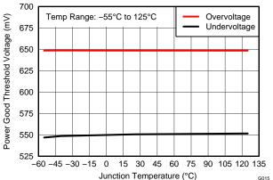
Figure 16. V<sub>OV</sub>/V<sub>UV</sub> Power Good Threshold Voltage
