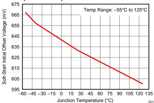
Figure 15. Soft-Start Initial Offset Voltage vs Junction Temperature
