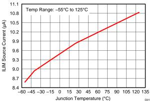
Figure 14. ILIM Source Current vs Junction Temperature
