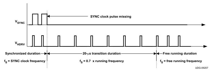
Figure 26. Transition for SYNC Clock Signal Missing (for Slave-180 Mode)
