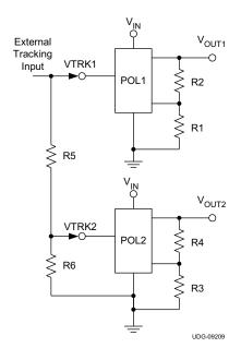
Figure 28. Simultaneous Voltage-Tracking Schematic
