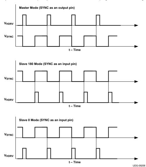
Figure 25. Frequency Synchronization Waveforms in Different Modes
