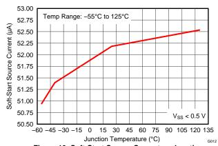
Figure 13. Soft-Start Source Current vs Junction Temperature ( $V_{SS} < 0.5 V$ )
