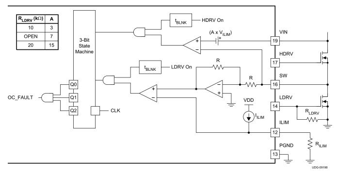
Figure 20. OCP and SCP Protection Functional Block Diagram
