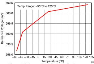
Figure 2. Reference Voltage vs Junction Temperature
