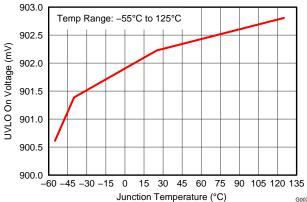
Figure 8. UVLO On Voltage vs Junction Temperature
