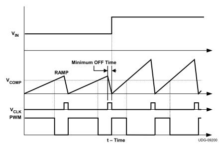
Figure 19. Feed-Forward Oscillator Timing Diagram
