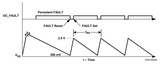
Figure 23. Overcurrent Fault Restart Timing
