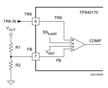
Figure 27. Tracking Functional Block
