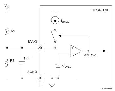
Figure 18. UVLO Functional Block Schematic
