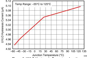
Figure 9. UVLO Hysteresis Current vs Junction Temperature
