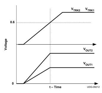
Figure 30. Ratiometric Voltage-Tracking Schematic Figure 31. Ratiometric Voltage-Tracking Waveform
