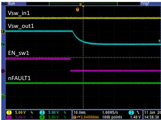
Figure 26. Power Switch1 Turn Off Delay and Fall Time R_{OUT} = 5\ \Omega , C_{OUT} = 22\ \mu\text{F}
