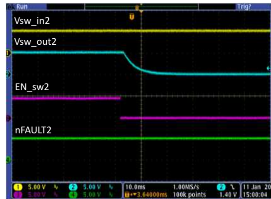
Figure 27. Power Switch2 Turn Off Delay and Fall Time R_{OUT} = 5\ \Omega , C_{OUT} = 22\ \mu\text{F}
