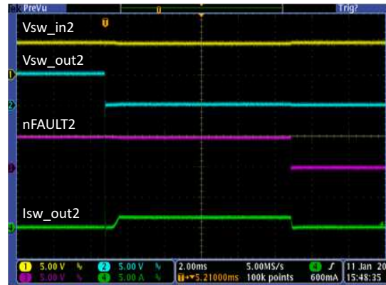
Figure 31. Power Switch2 Current Limit Operation
