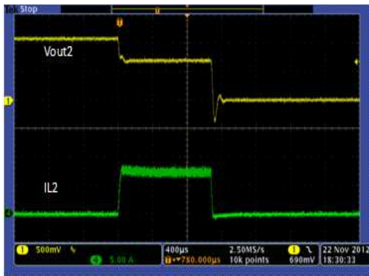
Figure 29. Over Current Protection, Buck 2
