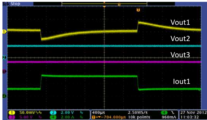
Figure 22. Transient Response Buck1@1.2V, 1-3A Step, C_o = 68\ \mu\text{F}
