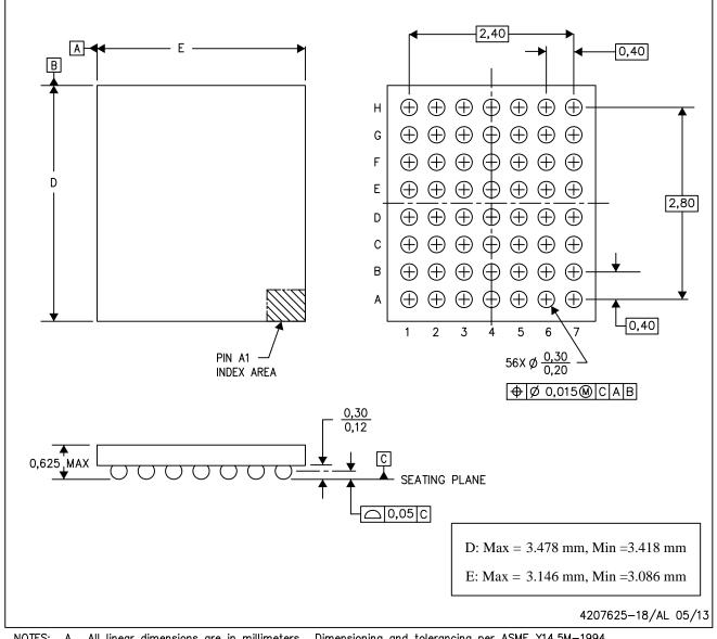
NOTES: A. All linear dimensions are in millimeters. Dimensioning and tolerancing per ASME Y14.5M-1994. B. This drawing is subject to change without notice.
