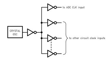
Figure 23. Isolating the ADC clock from other circuitry with a clock tree.
