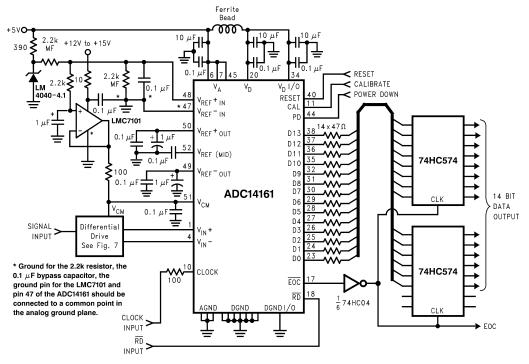
Figure 19. Simple application circuit with single-ended to differential buffer.
