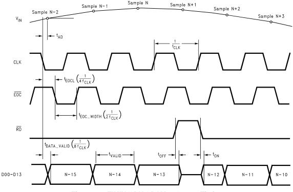
Figure 14. TIMING DIAGRAM 1. Output Timing
