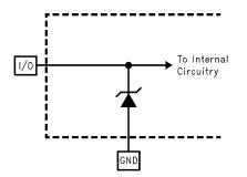
Figure 2. ESD Protection Scheme for Analog Input and Digital Output pins
