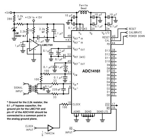
Figure 21. Driving the signal inputs with a transformer.
