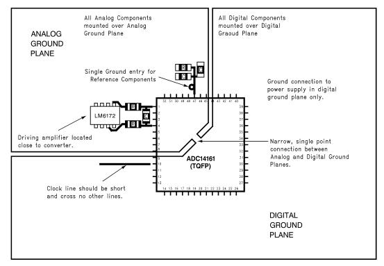
Figure 22. Example at a suitable layout
