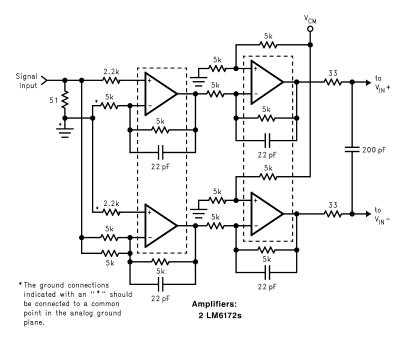
Figure 20. Differential drive circuit of Figure 19. All 5k resistors are 0.1%. Tolerance of the other resistors is not critical.
