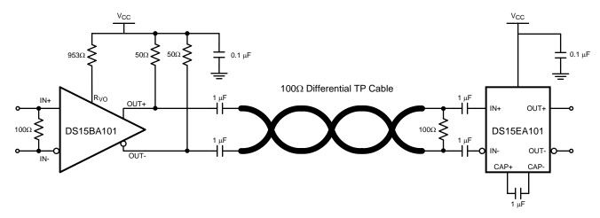
Figure 6. Cable Extender Chipset Connection Diagram for 100Ω Differential Cables
