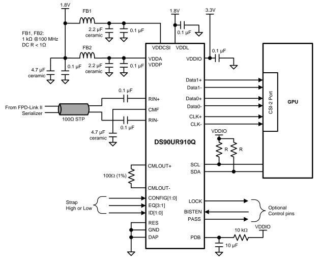
Figure 15. DS90UR910Q Typical Connection Diagram — Pin Control
