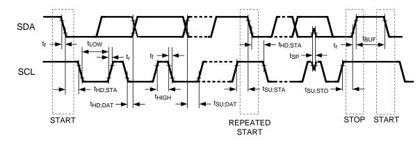
Figure 8. Serial Control Bus Timing Diagram
