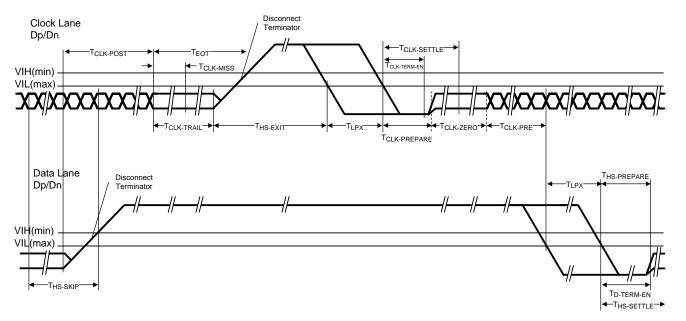
Figure 6. Switching the Clock Lane between Clock Transmission and Low-Power Mode
