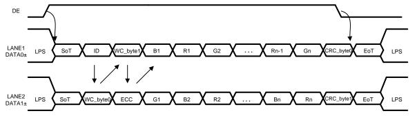
Figure 11. DATA0± and DATA1± packet format in according to CSI-2 protocol for RGB888
