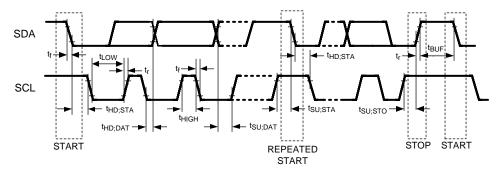
Figure 17. Serial Control Bus Timing Diagram
