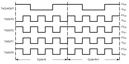
Figure 2. Checkerboard Data Pattern
