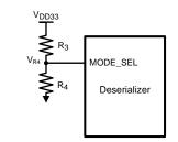
Figure 23. MODE\_SEL Connection Diagram
