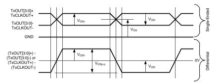
Figure 13. FPD-Link Single-ended and Differential Waveforms
