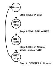
Figure 30. BIST Mode Flow Diagram
