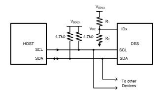
Figure 32. Serial Control Bus Connection
