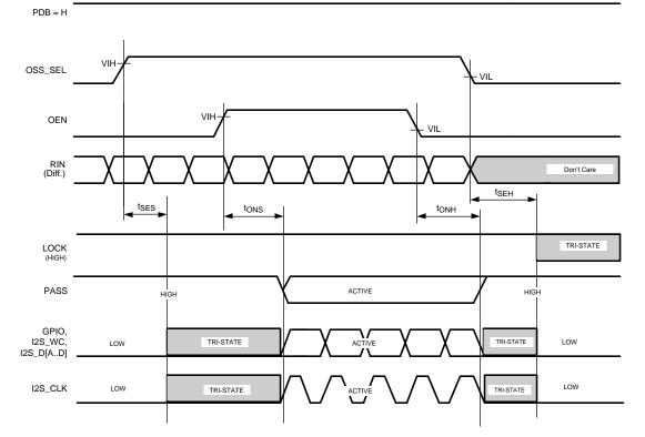
Figure 11. Output State (Setup and Hold) Times
