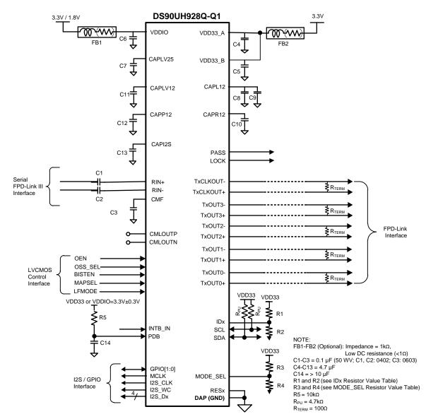
Figure 38. Typical Connection Diagram
