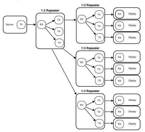
Figure 26. HDCP Maximum Repeater Application
