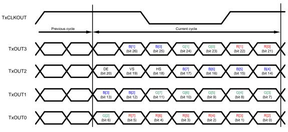
Figure 19. 24-bit Color FPD-Link Mapping: LSBs on TxOUT3 (MAPSEL=L)
