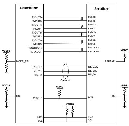
Figure 28. HDCP Repeater Connection Diagram
