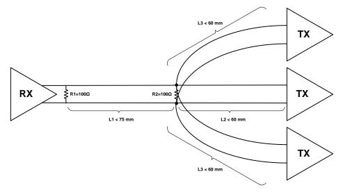
Figure 29. FPD-Link Fan-Out Electrical Requirements
