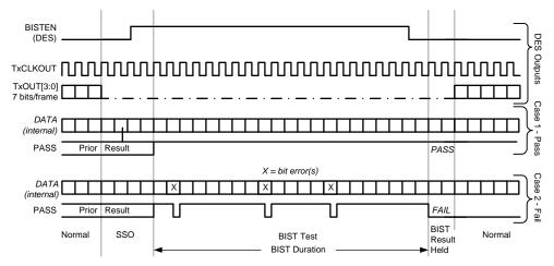
Figure 31. BIST Waveforms
