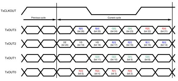
Figure 22. 18-bit Color FPD-Link Mapping (MAPSEL = H)
