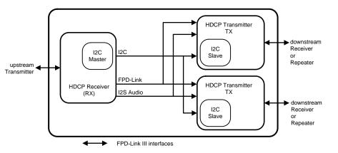
Figure 27. HDCP 1:2 Repeater Configuration
