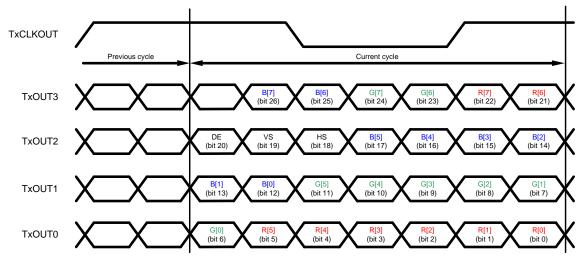
Figure 20. 24-bit ColorFPD-Link Mapping: MSBs on TxOUT3 (MAPSEL=H)
