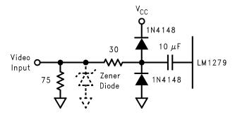
Figure 6. Recommended Video Input ESD Protection
