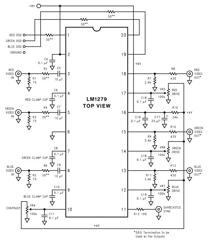
\*\***Note:** All video inputs *must* have a series 30Ω resistor for protection against EOS (Electrical Over Stress). If the OSD signals are external to the monitor, or these signals are present any time when +8V is not fully powered up, then the OSD inputs also *require* a series 30Ω resistor.
