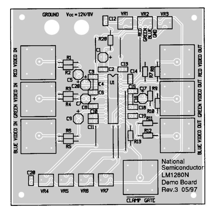
Figure 7. LM1279 OSD Video Pre-\Amp Demontration Board Layout
