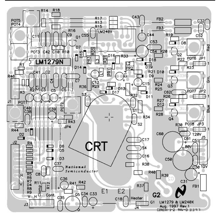
Figure 11. LM1279/LM2407 Demonstration Neck Board Layout
