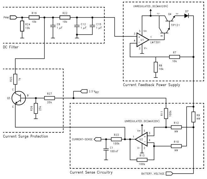
Figure 8. Circuitry Used for Li-Ion
