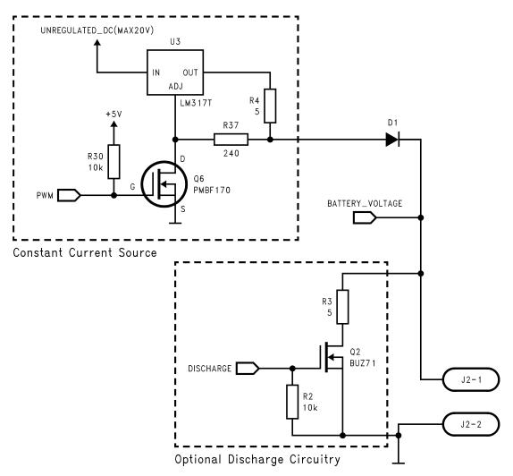
Figure 7. Circuitry Used Only for Ni-Cd/Ni-MH
