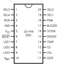
Figure 1. Top View See Package SOIC (DW)
