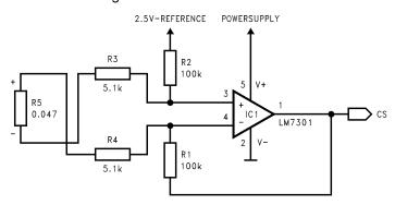
The current-sensing signal is amplified, inverted and centered on the 2.5V reference by the operational amplifier and fed into the CS pin on the LM3647. The amplification stage must be dimensioned by setting the appropriate ratio between R1 (R2) and R3 (R4). The figure above is dimensioned for a maximum current of about 1.1A. This was calculated using Equation 4:
