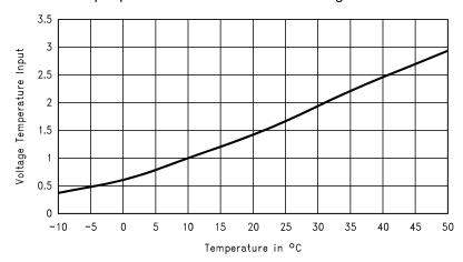
Figure 5. Typical Configuration Curve, (NTC Characteristics: 3 kΩ @ 25°C, β=3988)
