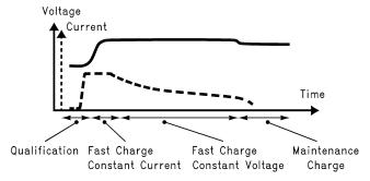
Figure 4. Li-Ion Charging Curve
