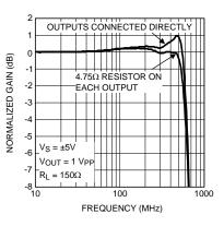
Figure 28. Input Expansion Frequency Response with Direct Connection and Isolation Resistors
