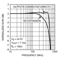
Figure 29. Input Expansion Frequency Response
