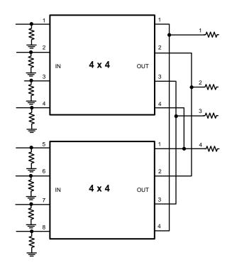
Figure 26. Input Expansion with Shared Termination Resistors
