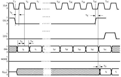
Figure 32. Timing Diagram for Serial Mode
