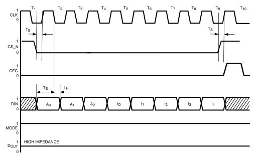
Figure 33. Addressed Mode Timing Diagram
