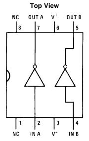
Figure 1. PDIP Package See Package Number P0008E
