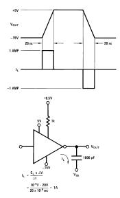
Figure 16. Clock Waveforms (Voltage and Current)
