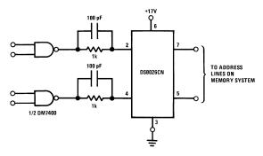
Figure 14. DC Coupled RAM Memory Address or Precharge Driver (Positive Supply Only)
