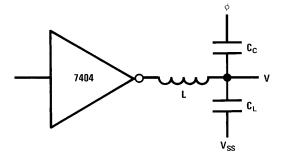
Figure 17. Clock Coupling
