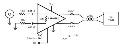
Figure 41. LMH6882 Used as Twisted Pair Cable Driver
