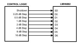
Figure 49. Parallel Mode Connection
