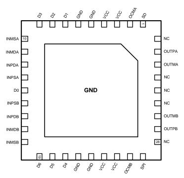
Figure 3. 36-Pin WQFN Top View
