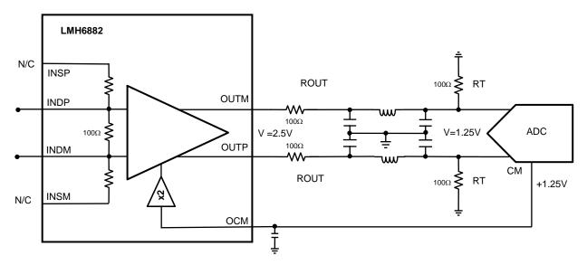
Figure 48. DC-Coupled ADC Driver Example 2, ADC12D1800RF with Terminated Input
