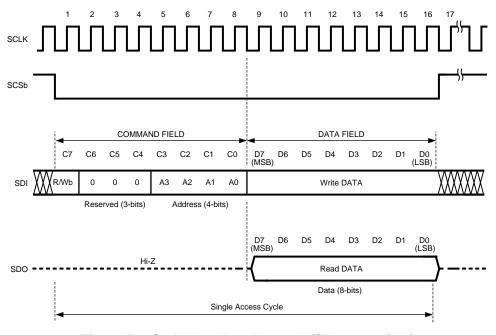
Figure 50. Serial Interface Protocol (SPI compatible)
