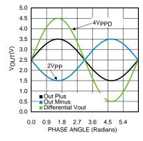
Figure 44. Differential Output Voltage
