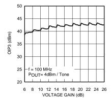
Figure 1. OIP3 over Voltage Gain Range
