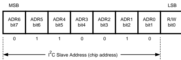
Figure 21. LP55231 Chip Address
