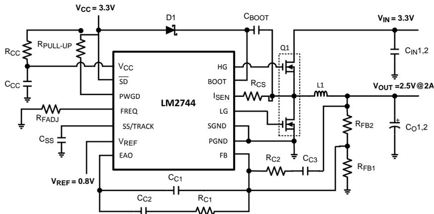
**Figure 36. 3.3V to 2.5V at 2A, V<sub>REF</sub> = 0.8V, F<sub>SW</sub> = 300kHz**
