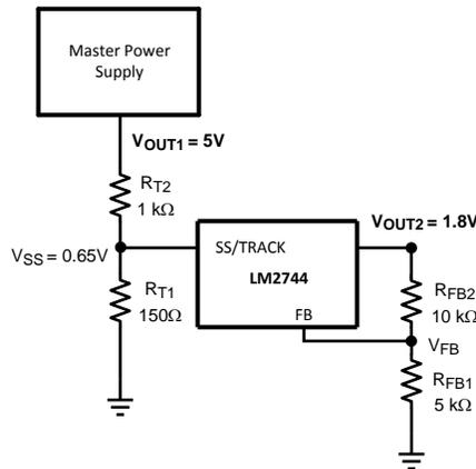
Figure 21. Tracking Circuit
