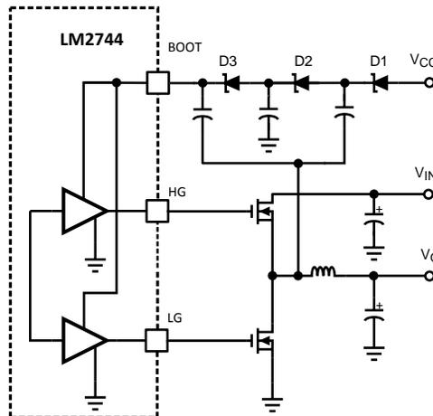
Figure 29. Charge Pump with Added Gate Drive
