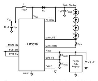
Figure 1. Main Display with OLED Sub Display
