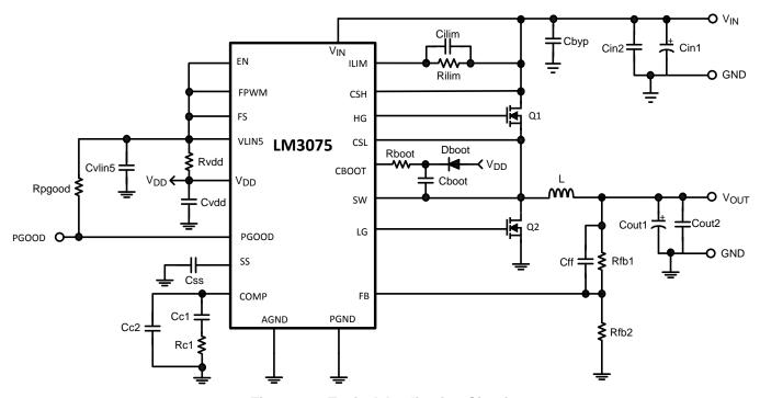
Figure 23. Typical Application Circuit
