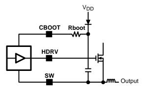
Figure 17. Adding a resistor in series with the CBOOT pin to suppress the turn-on switching noise
