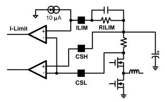
Figure 16. Current Sensing by External Sense Resistor
