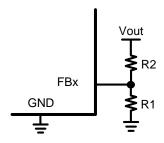
Figure 18. Output Voltage Setting
