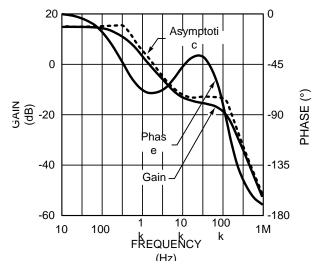
Figure 20. Control-Output Transfer Function
