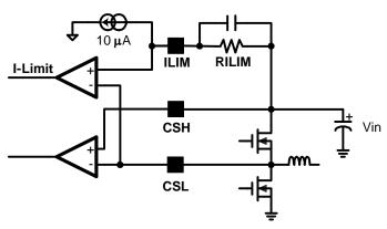
Figure 15. Current Sensing by Vds of the Top FET
