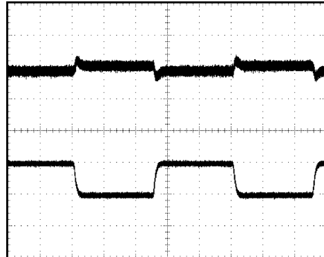
V_{IN} = 12V , V_{OUT} = 3.3V , I_{OUT} = 300\text{ mA to } 200\text{ mA to } 300\text{ mA} Top trace: V_{OUT} , 20 mV/div, AC Coupled Bottom trace: I_{OUT} , 100 mA/div, DC Coupled T = 200 \mu\text{s}/\text{div}
