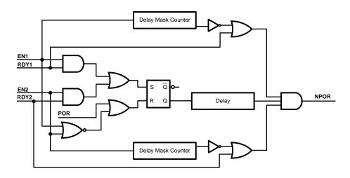
Figure 31. Design Implementation of the Flexible Power-On Reset
