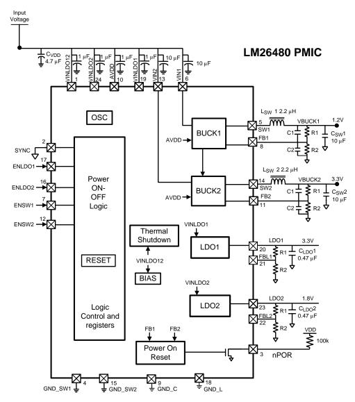
Figure 1. Application Circuit
