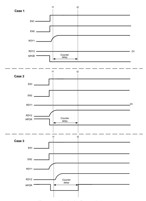
Figure 28. NPOR with Counter Delay
