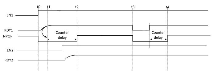
Figure 29. Faults Occurring in Counter Delay After Startup
