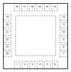
Figure 2. 24-Lead WQFN Package (top view)
